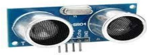
Gambar 2.7 Sensor Ultrasonik
