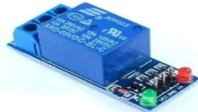
Gambar 2.11 Relay 1 Channel
